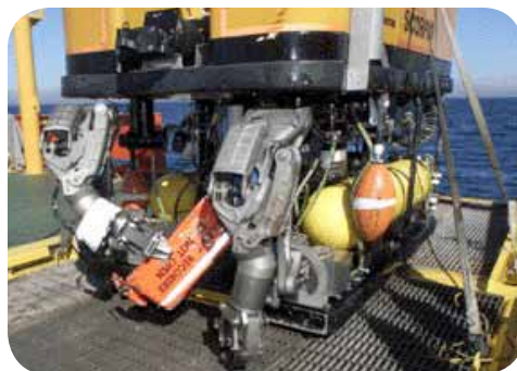
CONAN manipulators combine strength and dexterity.
